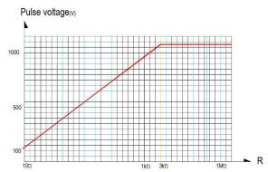
Pulse load rating in accordance with IEC 60115-1,4.27;  $10\mu$ s/700 $\mu$ s; 10 pulses loaded, for permissible resistance change  $\pm$ (0.5%+0.05 $\Omega$ )
